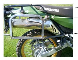
Rear mount M8x35mm SHCS Bolt, M8 Nylock nut, Nylon Spacer, 5/16" washers, and Turn Signal Tab
