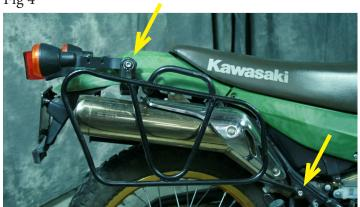
NOTE 1: The turn signal wiring has a factory supplied disconnect point hidden between the exterior (green color) and interior (black color) rear fenders. To take advantage of the supplied wiring disconnect you need to remove the exterior fender to access the wiring disconnect point.
