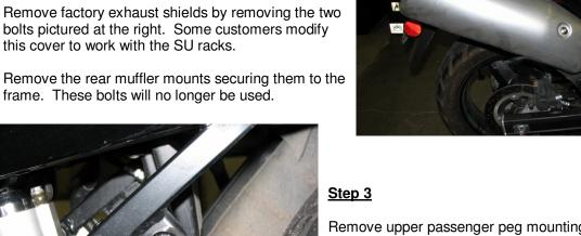
Remove upper passenger peg mounting bolts. It may also be helpful to loosen the lower mounting bolts to aid installation.
