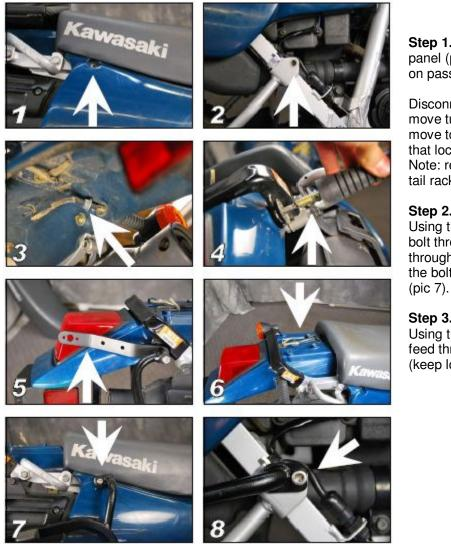
**Step 1.** Remove rear bolt on Side panel (pic 1) and rear (bolt) mount on passenger foot peg. (pic 2)
