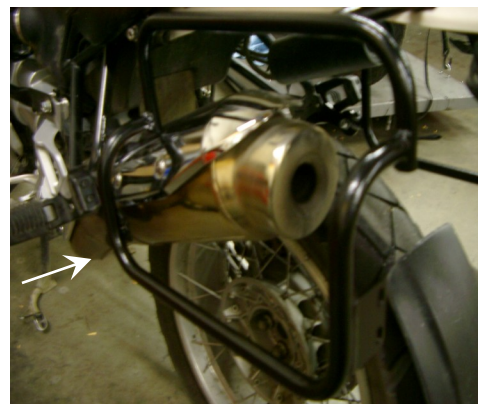
LOCATION WHERE THE MUFFLER AND HEADER MEET
