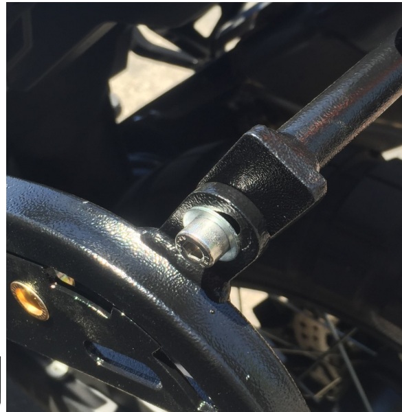
Figure 9: Rear SU Rack Mount
