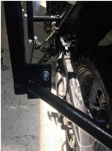
Figure 12.1: Bumper Mounts (Outside)
