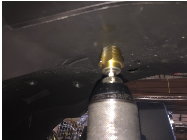
Figure 4: Picture shows holes being drilled in the inner plastic fender.
