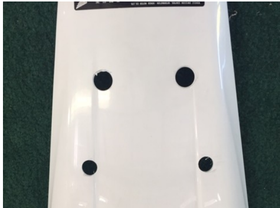
Figure 4: Holes drilled in fender cover.
