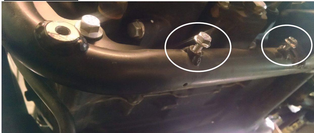
Step 5: Tighten head pipe nuts that you loosened in step 1 (see figure 7)
