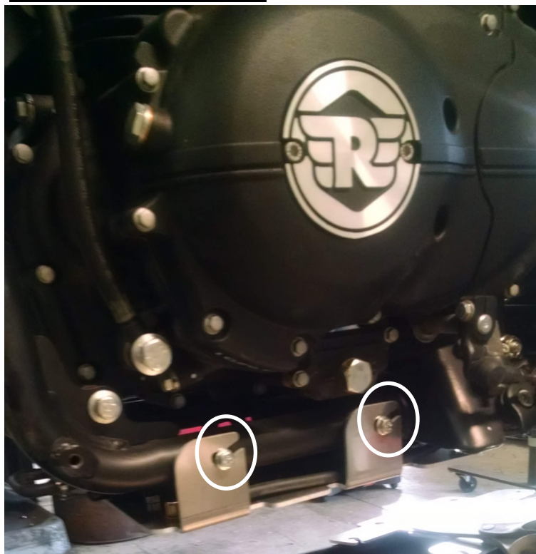
Figure 6 Base plate installed
