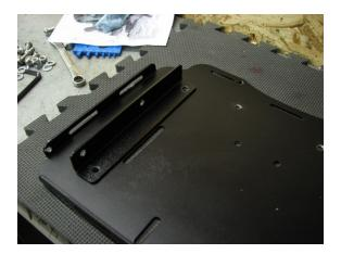
Note: The curved section of the tail plate faces the front of the motorcycle.
